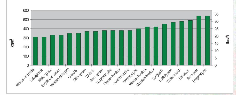
Source: USFS Forest Products lab (1999). Note: to convert kg/m<sup>3</sup> to Specific Gravity (SG), divide by 1,000. To convert kg/m<sup>3</sup> to lbs/ft<sup>3</sup>, divide by 16.
