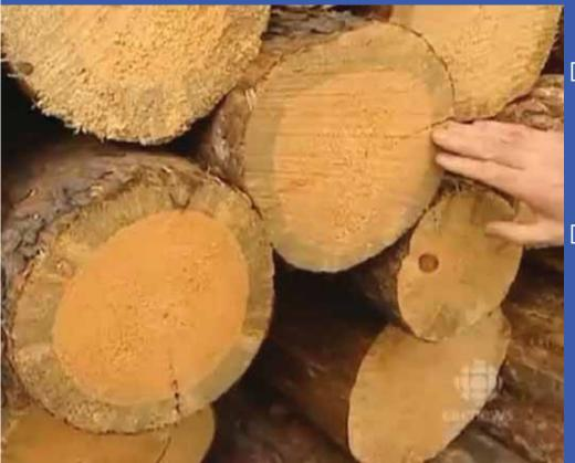
MPB killed LPP has.... **Blue Stain** Grading defect No volume reduction Surface Check(s) Result of moisture loss Common to have one Prominent check Defect volume reduction
